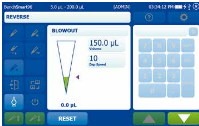
Figure 3-34: Reverse pipetting paused to dispense residual volume
