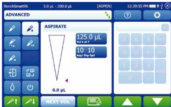
Figure 3-7: Selecting next volume in a sequence
