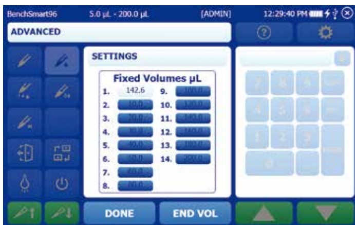
Figure 3-3: Setting one fixed volume
