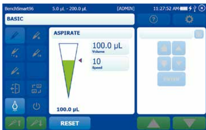
Figure 2-8: Screen depicting aspirated volume in tip
