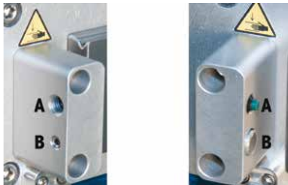
Figure A-3: Liquid head left stop bracket with stop A and magnet B
