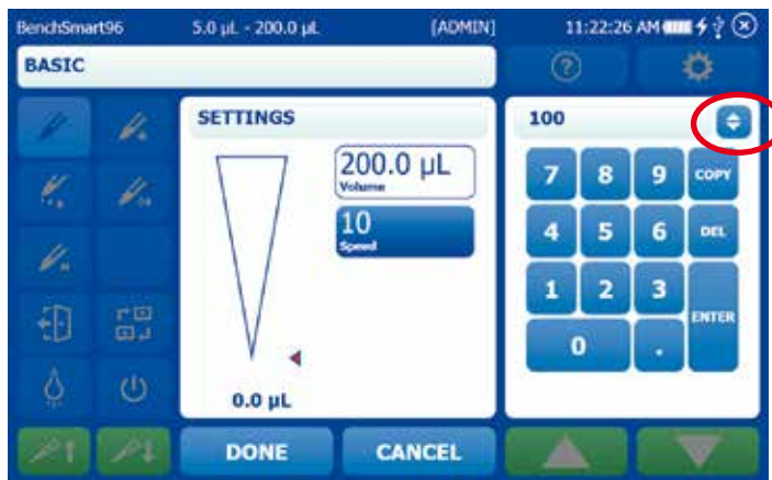
Figure 2-5: Setting the volume
