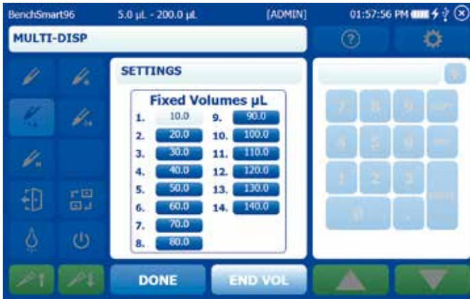
Figure 3-19: Setting one fixed volume
