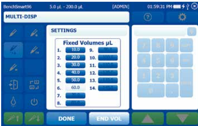
Figure 3-20: Setting a sequence of fixed volumes
