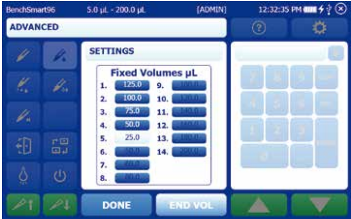
Figure 3-4: Setting a sequence of fixed volumes
