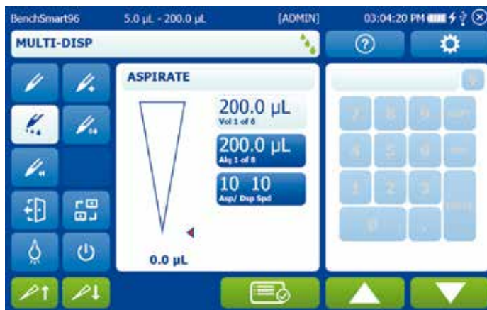
Figure 3-25: Sequential volumes greater than aspiration volume
