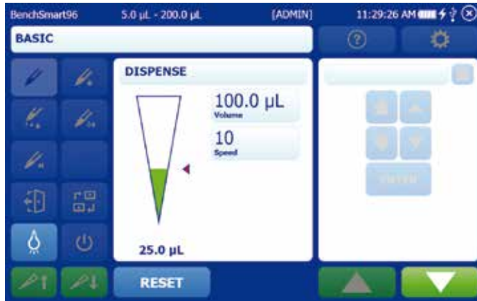
Figure 2-9: Screen depicting dispense volume in tip
