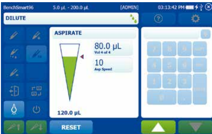
Figure 3-31: Sequential volumes in Dilute mode
