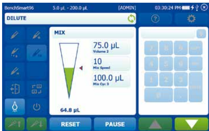
Figure 3-33: Mixing in Dilute mode
