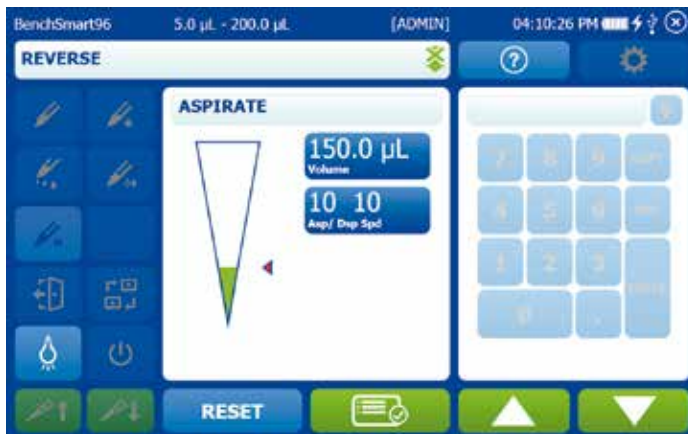
Figure 3-43: Reverse pipetting without "Blowout" option
