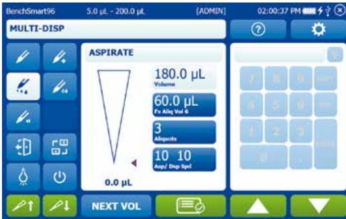
Figure 3-21: Selecting next fixed volume in series
