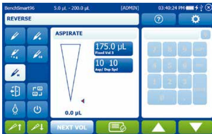
Figure 3-38: Selecting next fixed volume
