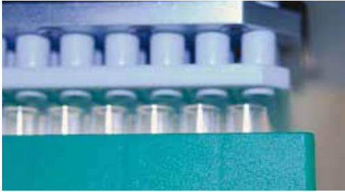
Figure A-2: Non-aligned nozzles (exaggerated view)
