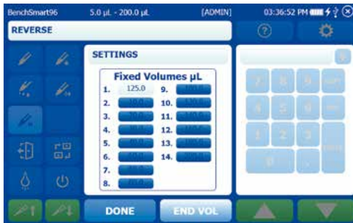
Figure 3-36: Setting one fixed volume
